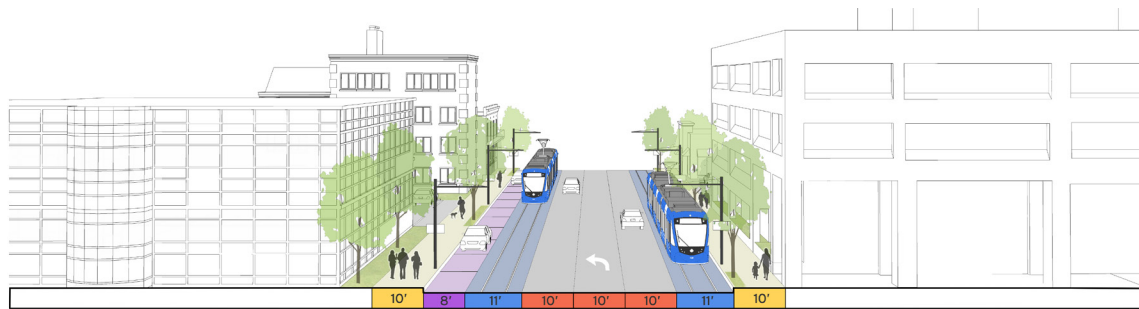
FIGURE 6.6 MAIN STREET WITH STREETCAR IN MIXED TRAFFIC, A LEFT-TURN LANE, AND A PARKING LANE
