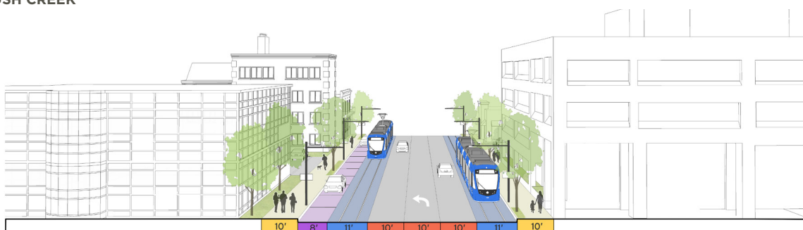
FIGURE 3.24 MIXED TRAFFIC STREETCAR WITH LEFT-TURN LANE AND ON-STREET PARKING SOUTH OF LINWOOD TO BRUSH CREEK
