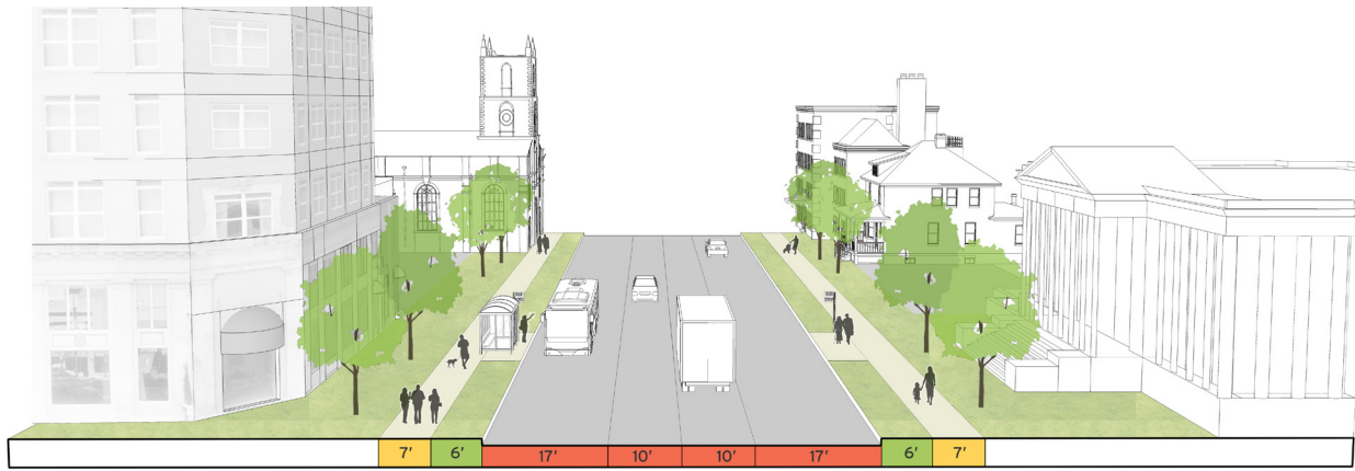
FIGURE 3.15 TYPICAL EXISTING SECTION ON LINWOOD BOULEVARD
